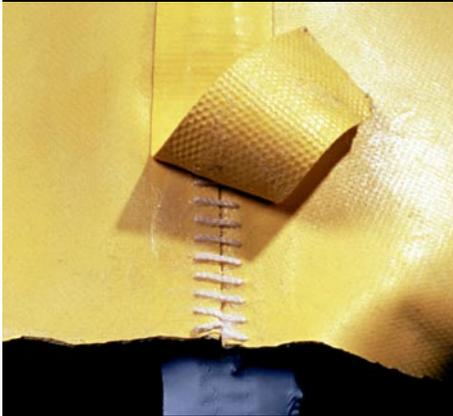
**TRELLCHEM HPS/VPS SEAM** Stitched with aramide thread for superior strength and durability. Taped with a rubber strip on the outside and a barrier laminate strip welded to the inside. This provides a continuous barrier layer across the seam.
